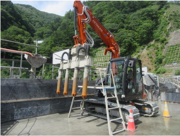
図-9 締め固め機械
